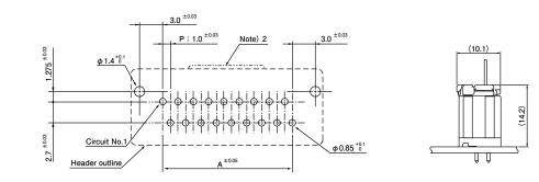
Note: 1. Dimension A in the above figure is the same as the dimensions A of the shrouded header.
