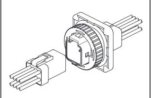
This is a panel lock type 2.0 mm pitch wireto-wire connector with water ingress protection with an IPX7 rating per IEC 60529 (grade 7 per JIS C 0920), suitable for use for the place of which waterproof is required.
