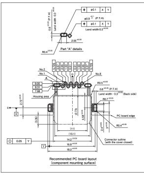
Note: 1. The PC board layout is the figure viewed from the connector mounting side.
