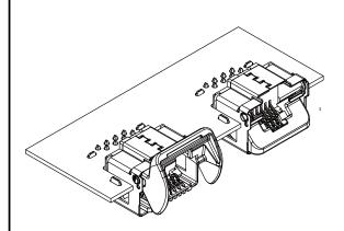
This is an interface connector compatible with RJ45 and designed as low profile and space saving type with a cover opening and closing structure.
