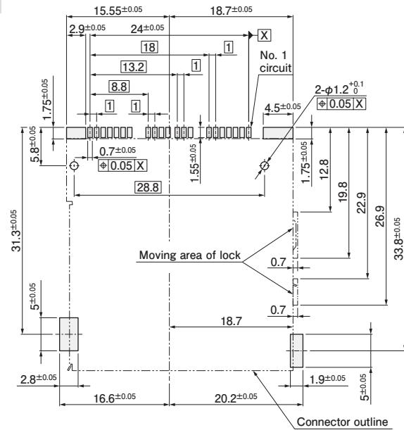
Note: 1. The PC board layout figure shown is viewed from the connector mounting surface.
